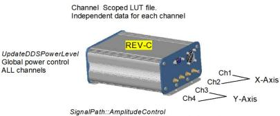
SignalPath::AmplitudeControl 4x Independent controls, one for each channel e.g. Ch1, Ch2 (X-axis) Ch3, Ch4 (Y-axis)
